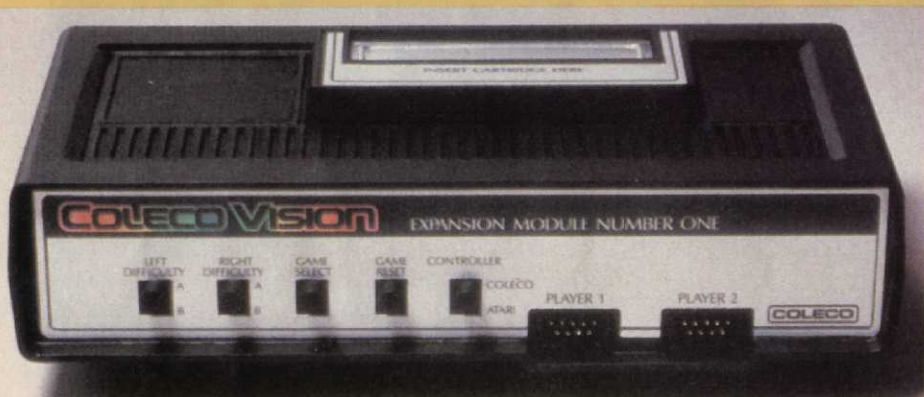
Coleco wants to render obsolescence obsolete with a series of expansion modules. The VCS adaptor, pictured above, will make VCS-compatible cartridges playable on ColecoVision.
